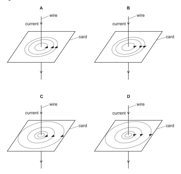
**39** The diagram shows a current-carrying wire in a magnetic field.
